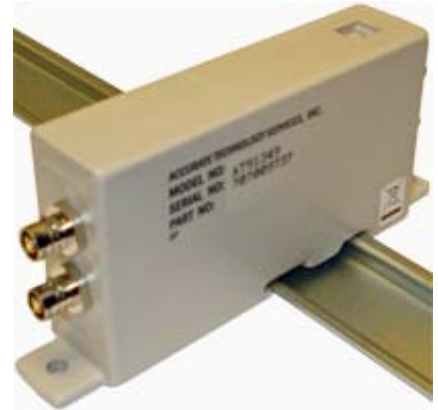
AT91349 shown mounted on 35 mm DIN rail
